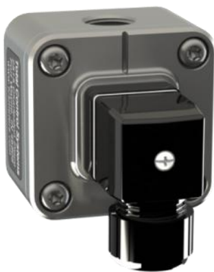
INSTALLED CORRECTLY: Face conduit entry downwards to avoid conduit moisture migration
